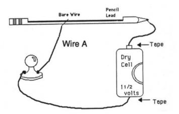
**Observations**: 1. What happens to the brightness of the bulb as you slide wire A along the lead?
